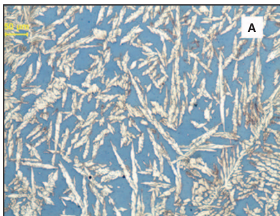
Fig. 5 — Micrographs of the FZ. A — Zone 1; B — Zone 3 (as-welded joint). Blue phase: ferrite; white phase: austenite; small white needles: secondary austenite.
