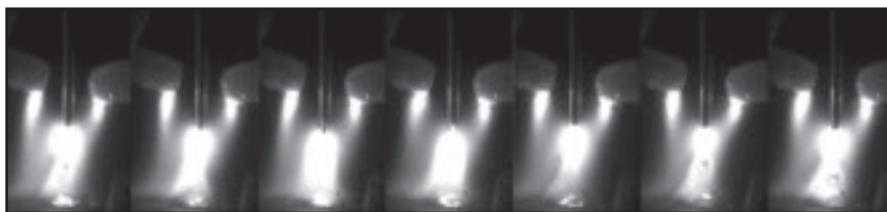
Fig. 14 — Metal transfer with dual 60-A bypass current in Experiment 5. The interval between each frame is 0.5 ms.
