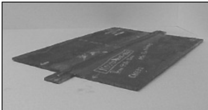
Fig. 6 — Gas metal arc welded plate.
