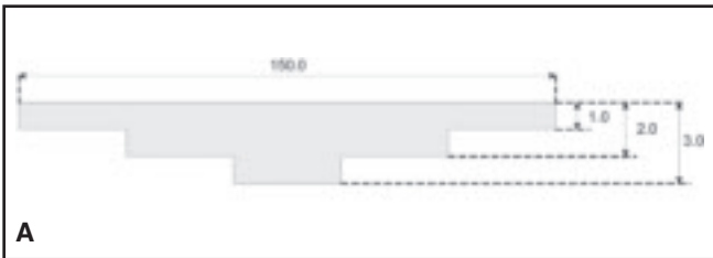
Fig. 7 — Profile of the three-dimensional part. A — Along the weld path; B — perpendicular to the weld path. All dimensions in mm.
