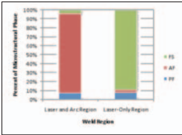
Fig. 4 — Weld metal microstructural content in the two different regions of the two-part fusion zone partial-joint-penetration welds.
