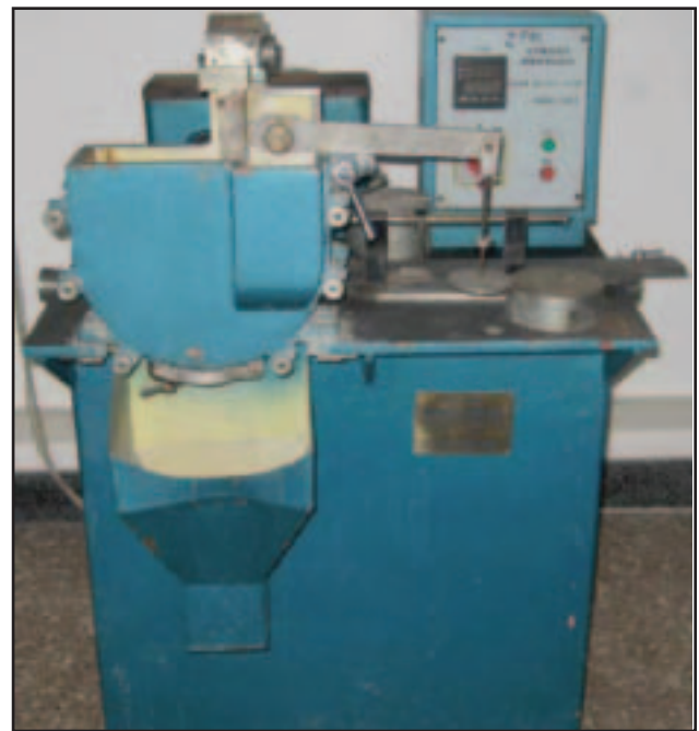
Fig. 4 — Abrasion test equipment (MLS-225 wet sand rubber wheel test machine).
