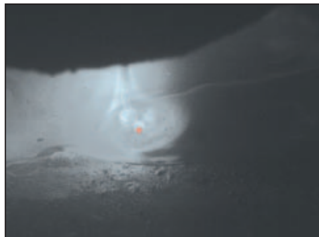
Fig. 12 — Weld pool image and weld pool surface center.
