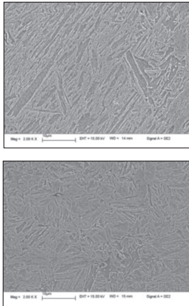
Fig. 13 — SEM views of the weld metal (top) and heat-affected zone (bottom) microstructures. The weld showed a completely martensitic structure. Isolated areas of ferrite and bainite were seen in the heat-affected zone. Nital-Picral etch.
