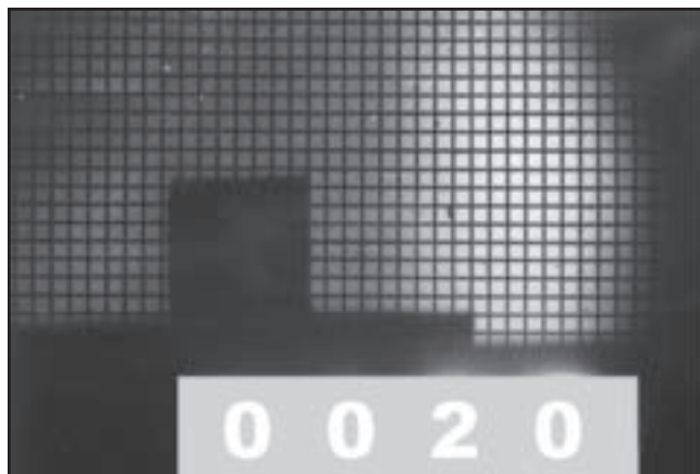
Fig. 1 — The contour of the specimen and temperature indication before heating test.
