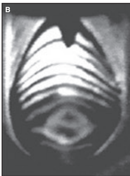
Fig. 1 — Captured images for weld pool measurement. A — 2-D measurement (Ref. 7); B — 3-D measurement (Ref. 8).
