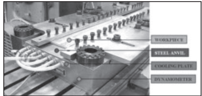
Fig. 2 — Setup of the dynamometer, cooling plate, and workpiece mounting.
