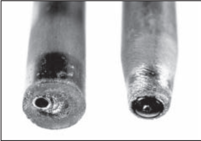
Fig. 5 — Images of 4.8-mm-diameter W-0.8% Zr electrodes after DSAW. The electrode on the right was ground to a 20-deg cone and truncated to 3.2 mm diameter and exhibits a larger molten spot after welding than the blunt electrode shown on the left.
