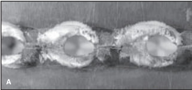
Fig. 7 — Top surfaces of welds made using a constant power of 2.6 kW and welding speeds; A — 10 mm/s with blowholes; B — good weld at 30 mm/s; C — inconsistent weld at 50 mm/s.
