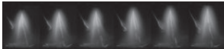
Fig. 17 — Smooth bypass metal transfer achieved with I_1 = 230\text{ A} and I_2 = 120\text{ A} .
