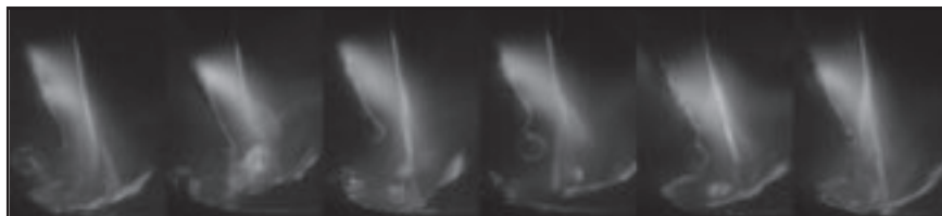
Fig. 18 — Smooth bypass metal transfer achieved with I_1 = 145\text{ A} and I_2 = 240\text{ A} .
