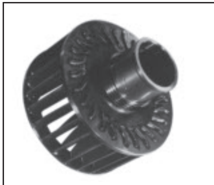
Fig. 1 — Titanium impeller brazed in vacuum at 890°C (1630°F) using Ti-24Zr-16Cu-16Ni (AWS BTi-4) filler metal (Design B).
