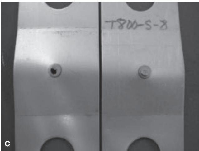
Fig. 10 — Different failure modes. A — Interfacial fracture; B — nugget pullout; C — partial interfacial fracture.
