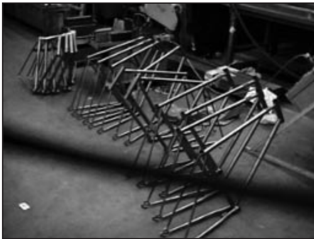
Fig. 15 — Fifteen bicycle frames prepared at Van Raam Aalten BV with five joined using each of the three brazing alloys: 70Cu-20Zn-10Mn, 54Cu-35Zn-6Ni-4Mn-1Si, and 44Ag-30Cu-26Zn.
