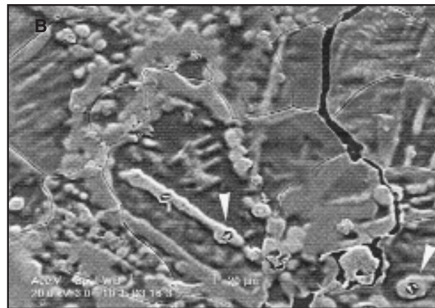
Fig. 5 — \delta -phase dissolution gradient in DRT specimens. A — As-received; B — 954°C/100 h treated condition (arrows indicate eutectic constituents formed in the cores of original \delta phase).
