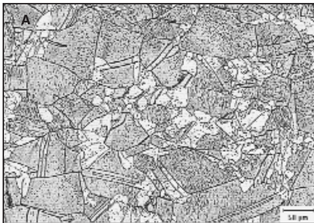
Fig. 1 — Microstructure of as-received Alloy 718 base metal: A — distribution of fine deformed grains at grain boundaries; B — short bar-shaped intra- and intergranular \delta phase.
