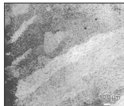
Fig. 8 — Fusion zone microstructure for specimen butt-joint welded using a welding current of 55 A.
