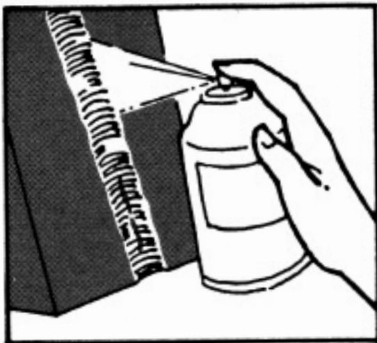
Fig. 9 — Developer is sprayed in 2 or 3 light applications, slightly damp on contact, from a distance of 8 to 12 inches.
