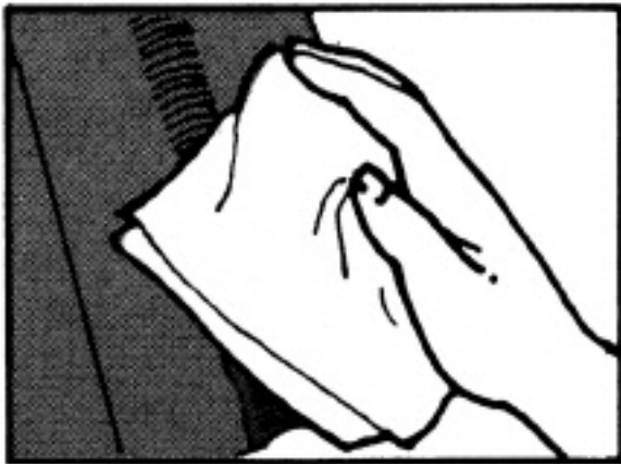
Fig. 5 — Surface penetrant is removed by wiping both with dry and with cleaner/remover moistened towels.
