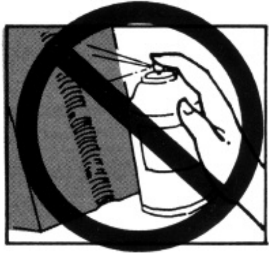
Fig. 8 — Avoid over-removal! Do not spray cleaner/remover directly on the surface to remove dye penetrant.
