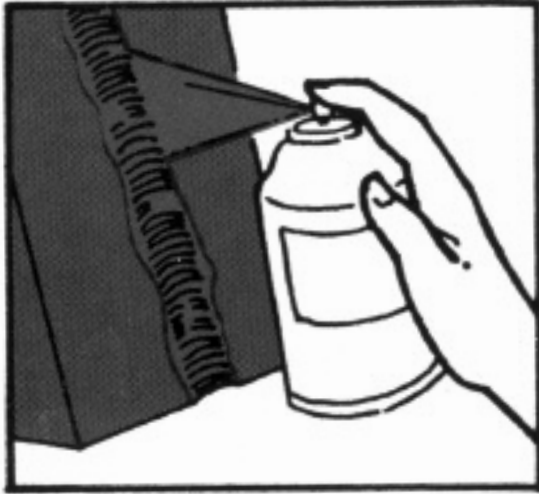
Fig. 3 — Cover the surface to be inspected with red dye penetrants.
