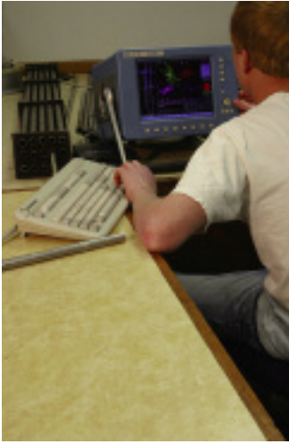
Justin James inspecting a heat exchanger mock-up with multi-frequency eddy current equipment. (Photo by Aaron Clark.)
