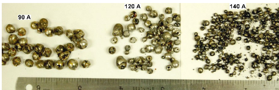
Figure 2. Droplets collected from E7018 electrodes melted with GTAW process using three welding current values (90, 120 and 140 A).
