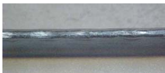
Figure 2. Appearance of weld beads in which the operational difficulties were overcome (conform weld over edge joint)
