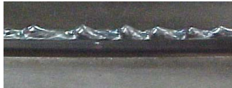
Figure 1. Appearance of a nonconformity weld bead, due to operational difficulties, over an edge joint using pure Ar melt-in Plasma process (the dragon's back shape is caused probably by over limit speed)
