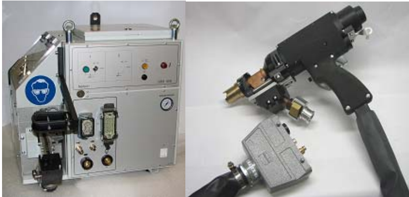
Figure 2. Stud feeder (left) and auto feed floating lift handgun (right)
