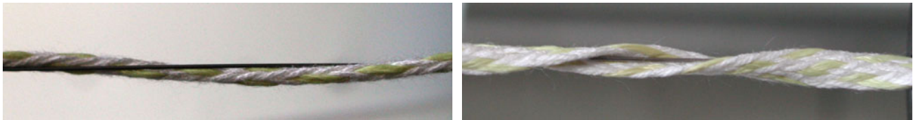
Picture 4: Braided round string (left) and flat, shoelace-like string (right) wrapped around a wire of diameter 1.2 mm
