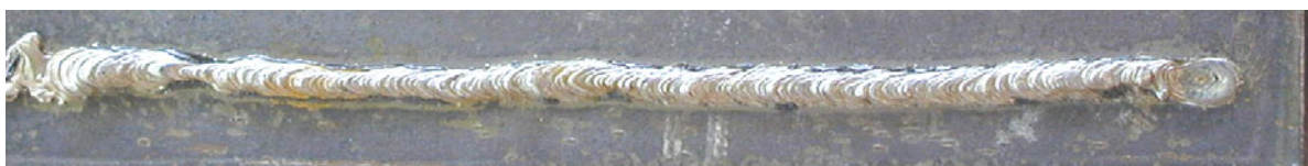
Figure 2 – Bead-on-plate wet weld deposited with E6013 electrode at 0.5 m water depth (the welding direction is from left to right-hand side).
