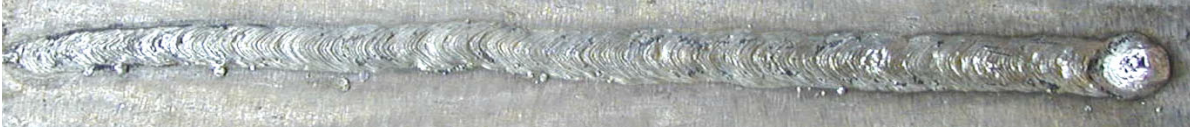
Figure 4 - Bead-on-plate wet weld deposited with E6013 electrode at 100 m water depth (the welding direction is from left to right-hand side).
