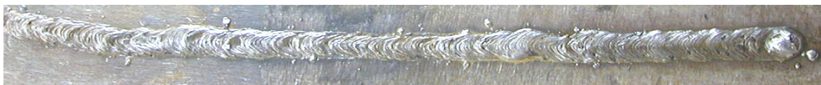
Figure 3 - Bead-on-plate wet weld deposited with E 6013 electrode at 50 m water depth (the welding direction is from left to right-hand side).
