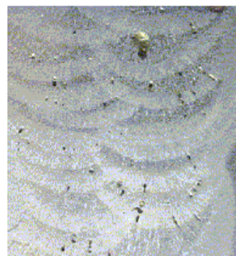
Figure 5 – V-groove weld with uniform pore distribution.
