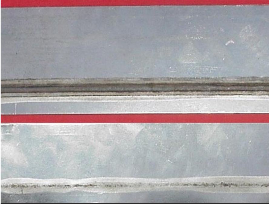
Figure 2 – Black soot on backside of the GMA-Pulse braze weld caused by excessive heat input (top). Significant reduction in the amount of zinc removed as a result of using Variable Polarity GMA brazing (bottom).
